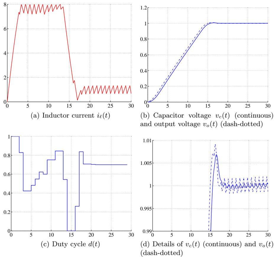
**Fig. 3.** Step response of the converter in nominal operation
