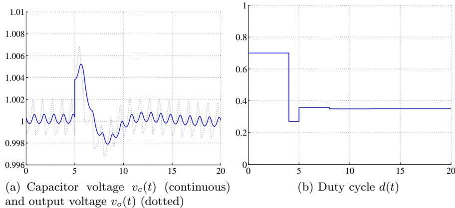
**Fig. 4.** Response of the converter to a step change in the input voltage from  $v_s = 1.5$  p.u. to  $v_s = 3$  p.u. at time-instant  $k = 4$
