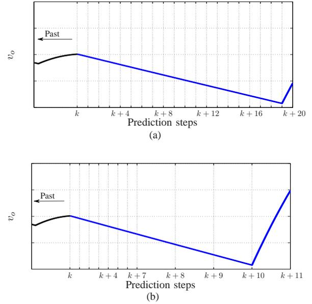
Fig. 6. Effect of the move blocking scheme. In (a), without move blocking, a prediction horizon of  $N = 20$  steps of equal time-intervals is needed. In (b), with the move blocking strategy employed, an  $N = 11$  prediction horizon is sufficient to achieve the same closed-loop result ( $N_1 = 7$ ,  $N_2 = 4$ , and  $n_s = 4$ , total length  $23T_s$ ).
