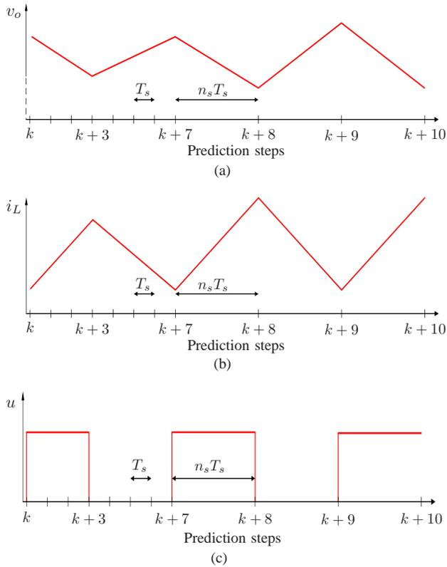
Fig. 5. Prediction horizon with move blocking: a) output voltage, b) inductor current, and c) control input. The prediction horizon has  $N = 10$  time-steps, but the prediction interval is of length  $19T_s$ , since  $n_s = 4$  is used for the last  $N_2 = 3$  steps.
