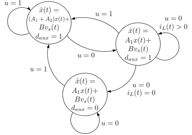
Fig. 2. Dc-dc converter presented as a continuous-time automaton.
