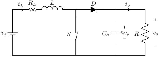
Fig. 1. Topology of the dc-dc boost converter.
