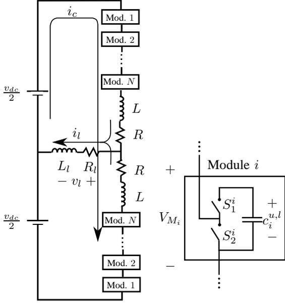
Fig. 1. Typical single-phase MMC configuration with  $N$  modules per arm.  $V_{dc}$  is the DC input voltage and  $v_l$  the voltage of the load (output)
