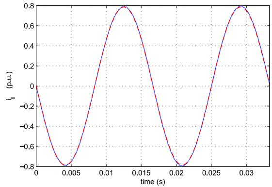
(f)  $i_l$ , Reference for the load current. The dashed line represents the reference ( $i_l = 0.8, \phi = 1.57$ ) see (1)
