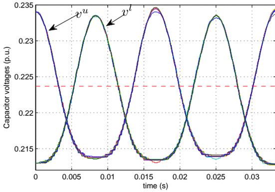
(c)  $v_l$  and  $v_u$ , Simplified DC reference for the voltages of the capacitors. The dashed line represents the reference ( $v_{DC}^{u,l} = 0.224$ )
