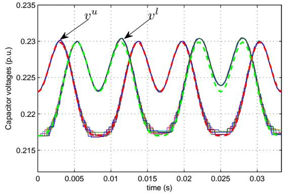
(d)  $v_l$  and  $v_u$ , Proposed reference for the voltages of the capacitors. The dashed lines represent the references see (28) and (29)
