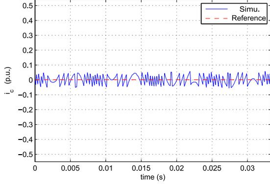
(a)  $i_c$ , Simplified DC reference for the circulating current  $i_c$ . The dashed line represents the reference ( $i_0 = 0.0014$ )
