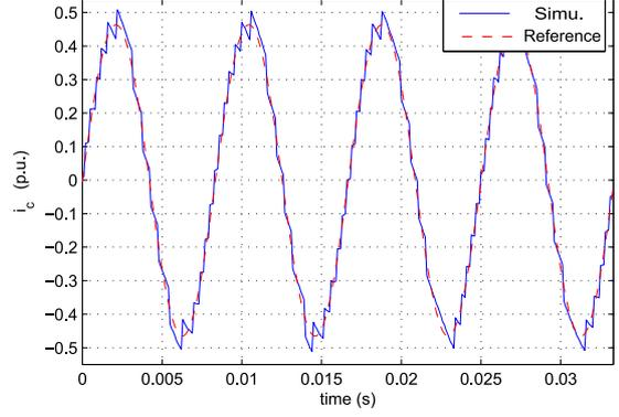
(b)  $i_c$ , Proposed Reference for the circulating current. The dashed line represents the reference ( $i_0 = 0.0014, i_2 = -0.46, \phi_2 = 1.6$ ) see (26)
