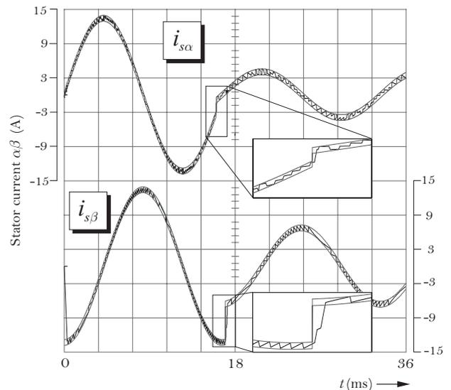
Fig. 5: Current trajectories with a bound width of 1.0A and reference changes
