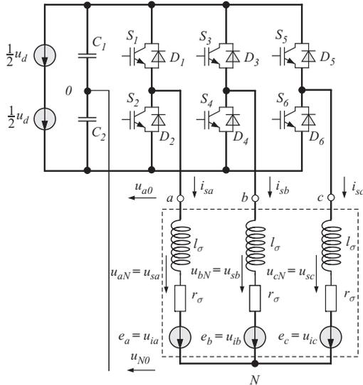
Fig. 1: Voltage Source Inverter driving an induction motor.
