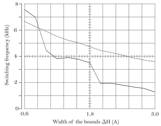
Fig. 4: Relationship between switching frequency and bound width.
