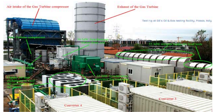
Figure 13: Test setup showing drive system, load generator, resistor bank and gas turbine
